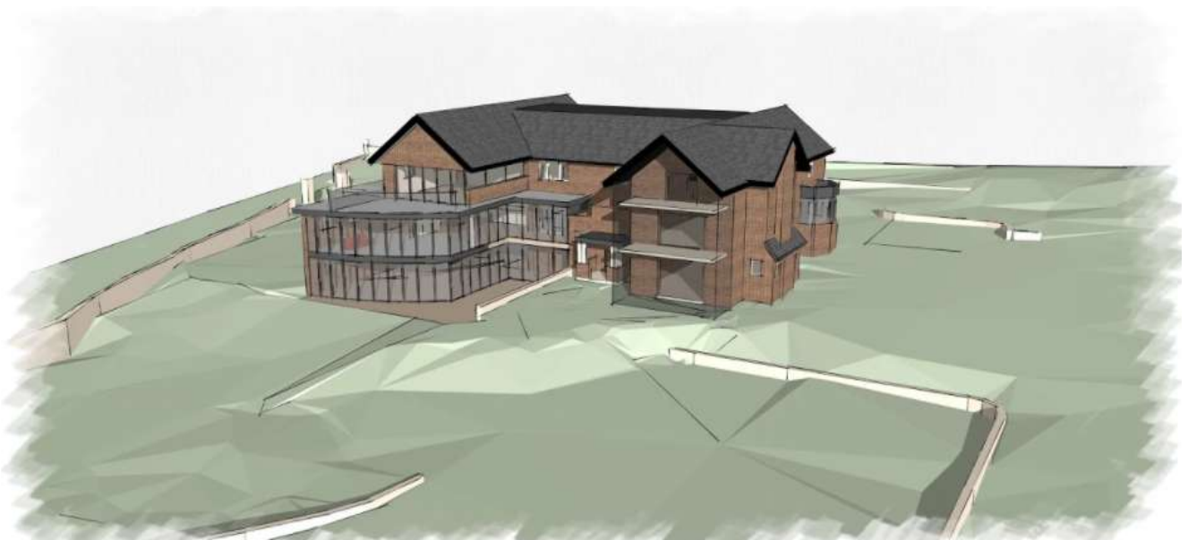
Figure 7. A steel framed structure allows for the installation of the specialist framed faceted glass feature wall which extends across two floors, providing views out at lower ground floor and ground floor levels
